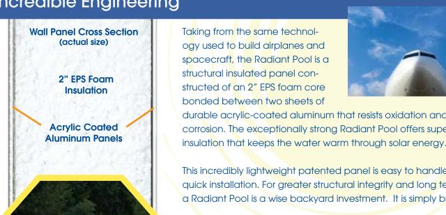
ogy used to build airplanes and spacecraft, the Radiant Pool is a structural insulated panel constructed of an 2" EPS foam core
