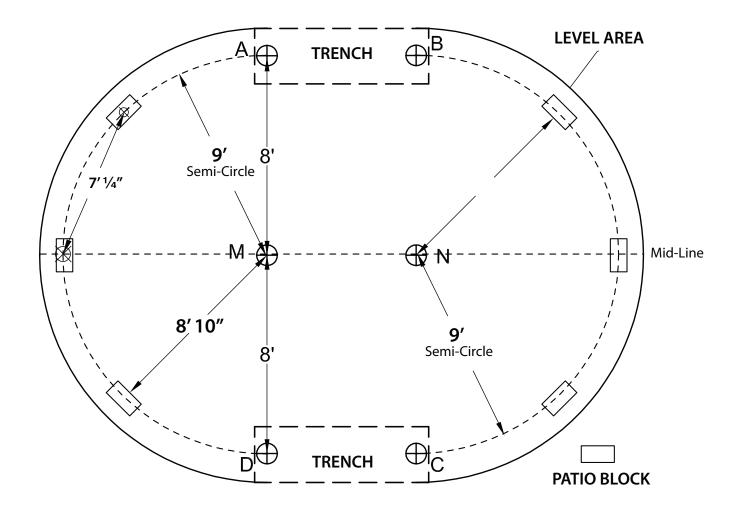
All radius panels will join near the center of the patio blocks.
