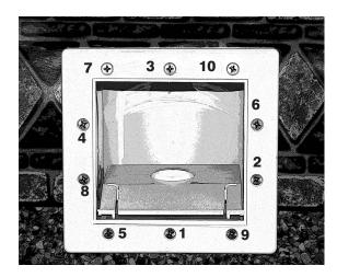
Skimmer faceplate installed w/screw tightening sequence.
