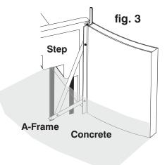
**NOTE:** Complete backfill is required around the step.
