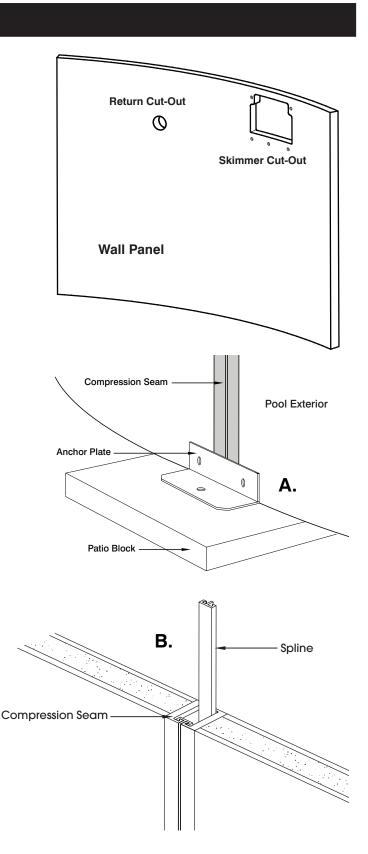
NOTE: Do not install final radius panel until after installing a-frames and sand has been brought inside pool.
